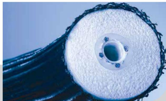
The special way in which the heating conductors are processed into the hose braiding optimizes the heat transfer. This means that, even with severe bending or torsional movement, contact between the heating conductors and the surface of the hose will be ensured at all times, and prevents overheating (also referred to as "hot spots"). Damage to the heating
