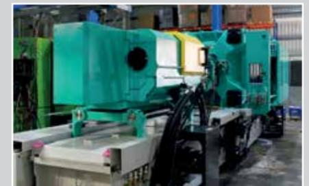
CNC-controlled injection moulding machine. Temperature-controlling the plastic and adhesive in the heated hose during manufacture of housing parts (PA, TPE, EVA). Temperature of medium: +90°C to + 180°C
