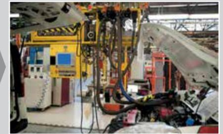
Wax-conveying hoses, heating capacity 60-120 W/m. Heating with minimized tolerances to guarantee extremely uniform consistency
