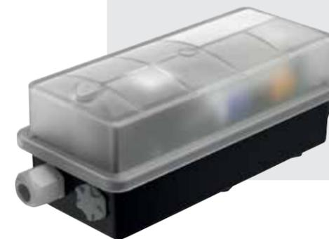
**templine®-B** Electronic temperature controller with integrated temperature limiter (safety temperature limiter). PI control characteristic, system deviation +/- 1K. Sensor input: PT100, two/three conductor technology. Switching capacity: 1360 VA/ 6A
