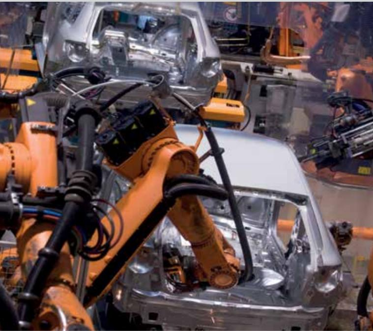
In automobile production, robots coat body parts with a fluid wax preservation coating
