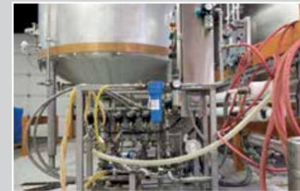
Flexible connection by heated hoses between tank and production installations. Maintaining temperature and compensating for vibrations along the conveyance path
