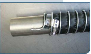
5. Bend the metal clip profile forward at a 90° angle to the hose.
