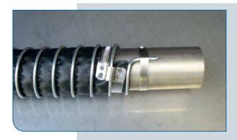
As is shown in images 8 - 9, the metal clip profile sits on the pipe and is fixed in place by the separate clamp, metal on metal. This type of connection is recommended. Other methods of grounding are also possible, however, we would like to point out the following:
