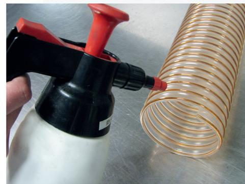
3. Clean the inner thread of the PU screw connector thoroughly and remove any dirt or grease
