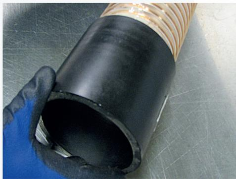
6. Carefully and evenly screw the PU part onto the end of the hose, which has just been prepared with the adhesive
